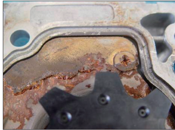
Bottom plate corrosion
